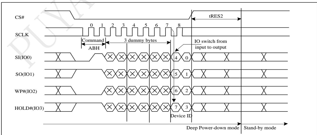
**Figure 10-42b Release from Deep Power-down (RDP) Sequence (Command AB)**
